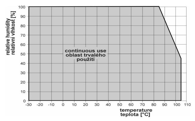
Measuring temperature and humidity range is limited in accordance with the graph below!
